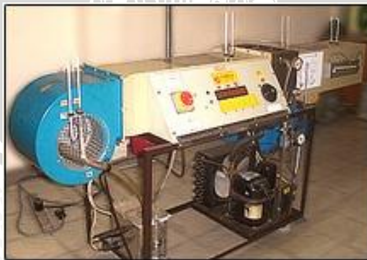
Gambar 3.1 Instalasi AC Bench PA Hilton
