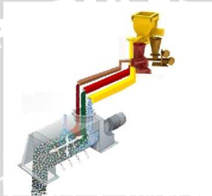
**Gambar 2.2** Ilustrasi *Continuous Mixing*
