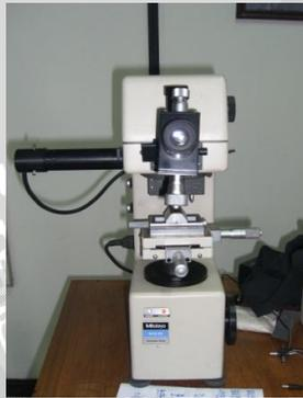
Gambar 3.15 : *Micro Vickers Hardness Tester type Mitutoyo MVK-E3*
