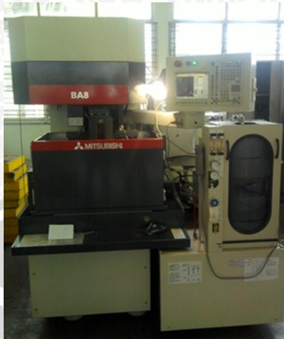
Gambar 3.1: Mesin Wire EDM Mitsubishi BA-8
