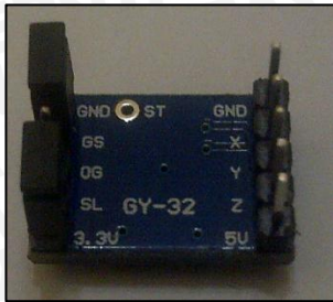
Gambar 5 Accelerometer MMA7455 3-Axis Accel Module
