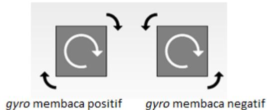
Gambar 4 Gyroscope sensor GS10 principle
