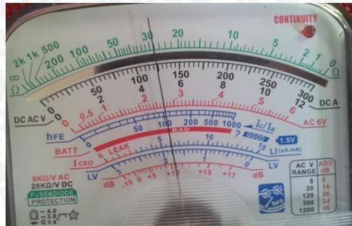
$I_B = 1,2 \text{ mA}$ . Skala 3 mA
