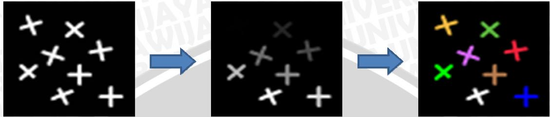
**Gambar 2.4** *Connected component labeling*
