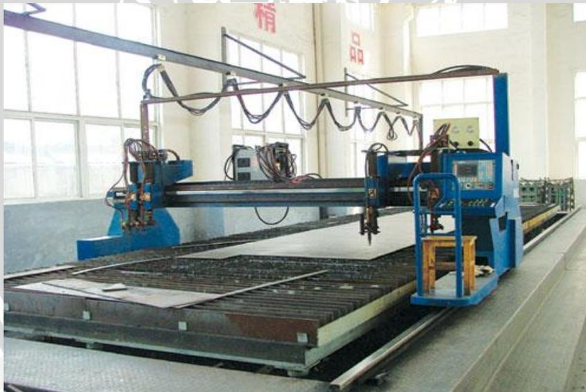
Gambar 3.1 Mesin *Plasma arc cutting*
