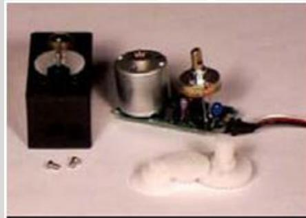
**Gambar 2.8** Sistem Mekanik Motor Servo
