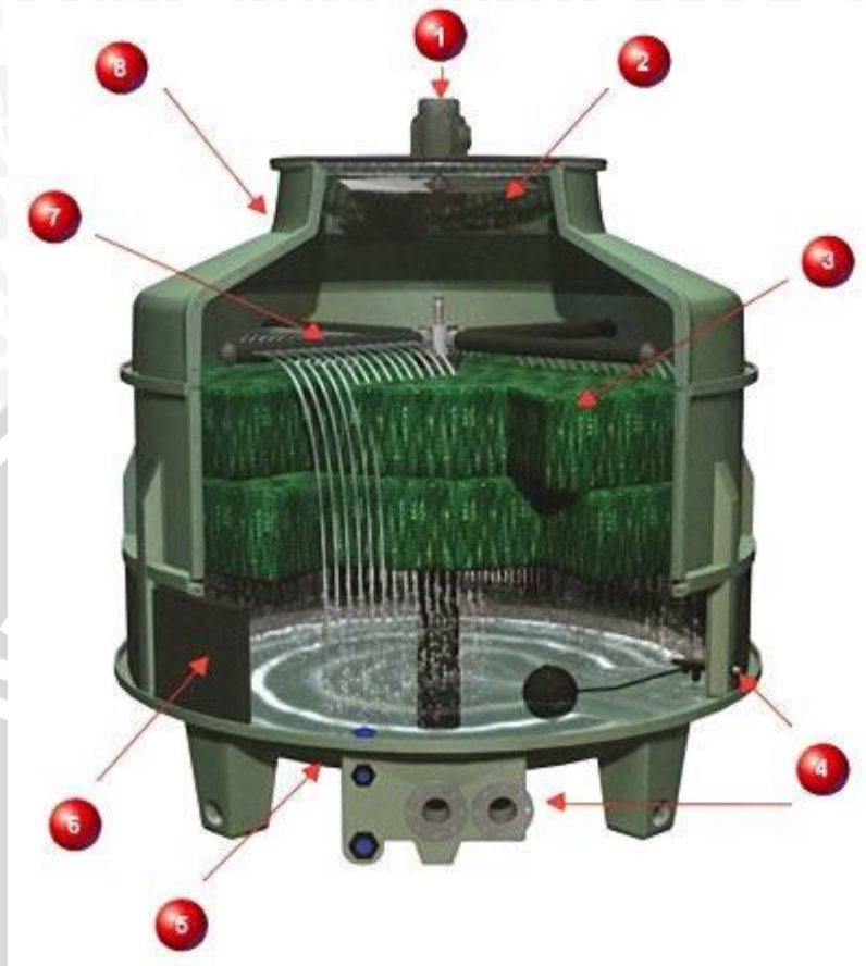
Gambar 2.2 : Bagian – bagian cooling tower Sumber :Southwest Thermal Technnology Inc. (n.d)
