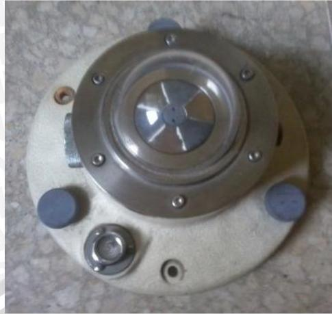
Gambar 3.3 Pyranometer
