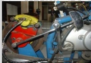
Gambar 3.5 *Dynamometer Prony Brake*
