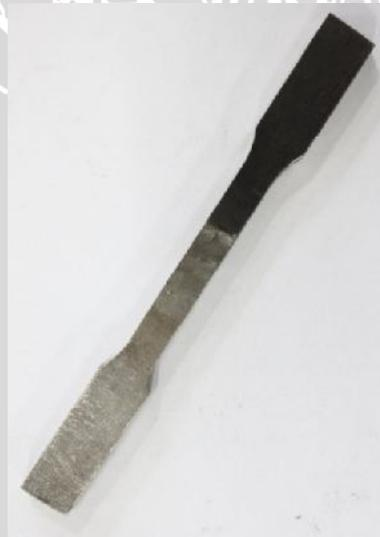
Gambar 4.1 Foto spesimen uji tarik standar ASTM A370
