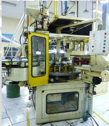
Gambar 2.23 *T.E.T (Heading Machine)*
