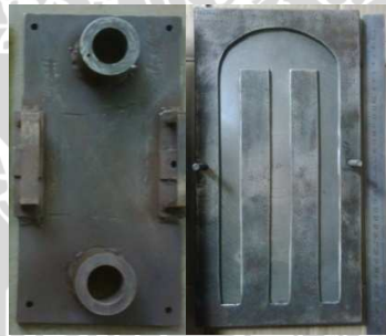
Gambar 2.3 Permanent Mold Casting Sumber: Laboratorium \alpha\beta , Landung sari-Malang
