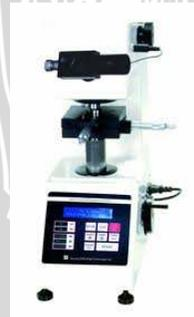
Gambar 3.8 Micro Hardness Tester
