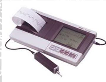
Gambar 3.5 Surface Roughness SJ 301
