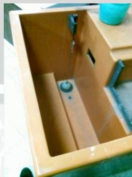
Gambar 3.6: Bak penampung (Hydraulic Bench).
