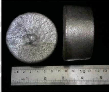
Gambar 3.10 *Ingot* Aluminium
