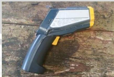
Gambar 3.6 *Infrared thermometer*
