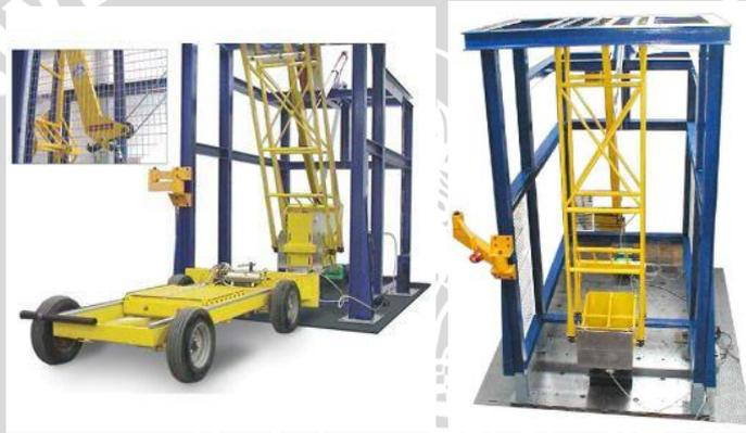
Gambar 2.7 Peralatan uji pendulum impak bumper
