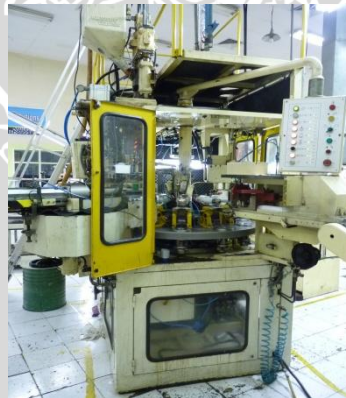
Gambar 2.24 T.E.T (Heading Machine)
