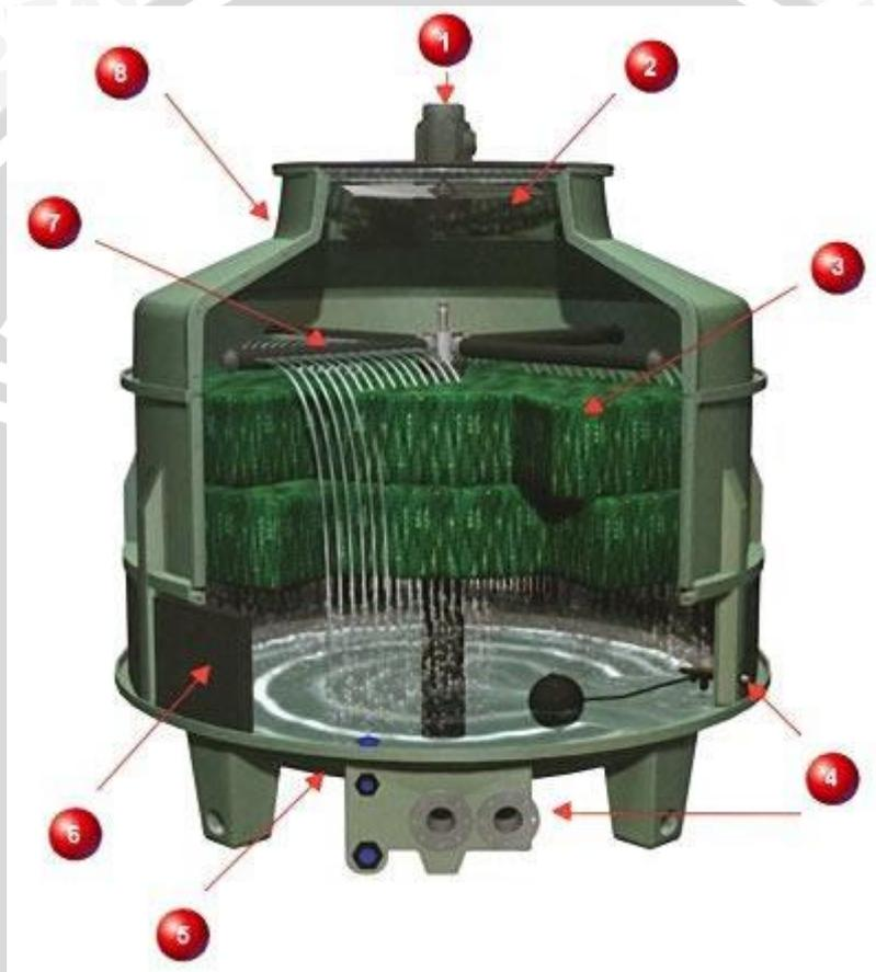
Gambar 2.2 : Bagian – bagian *cooling tower*
