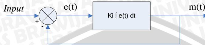
**Gambar 2.2** Diagram Blok Kontroler Integral
