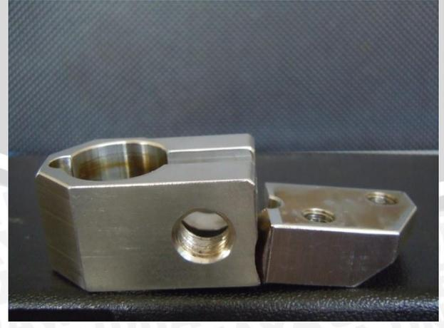
Gambar 1.5 Gambar *Gripper* Tampak Samping
