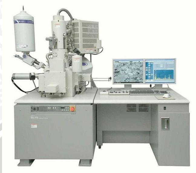
Gambar 3.2 *Scanning Electron Microscope* (SEM)
