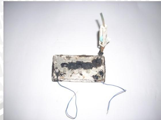
Gambar 3.1 *Microcombustor*
