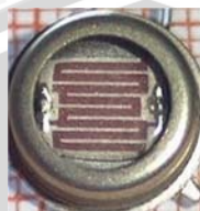
Gambar 2. 7 LDR ( Light Dependent Resistor ) Sumber: robotron-umm.blogspot.com
