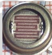
Gambar 2. 7 LDR ( Light Dependent Resistor ) Sumber: robotron-umm.blogspot.com
