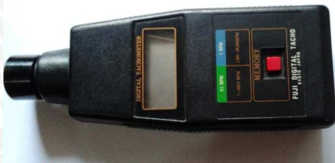
Gambar E. Digital tachometer
