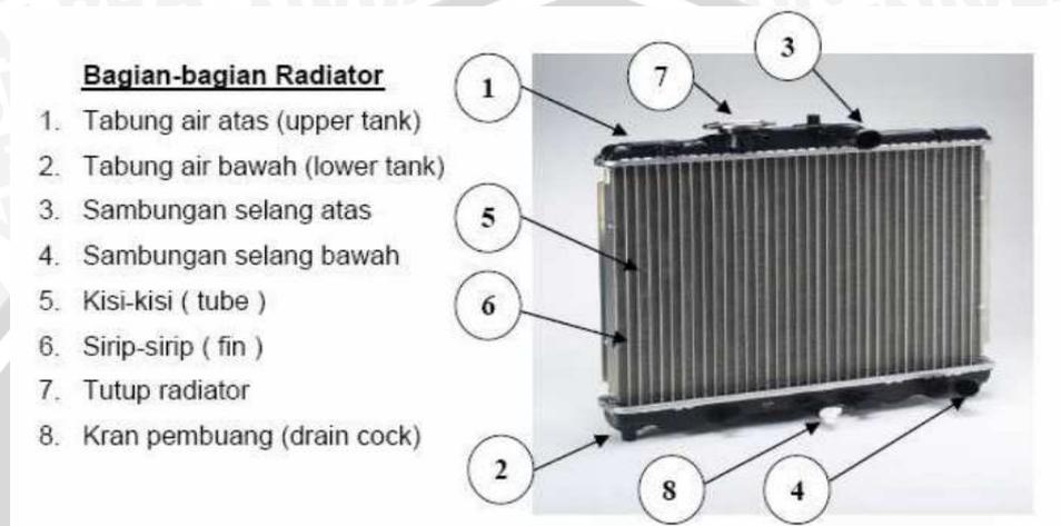
Gambar 2.2 Bagian-bagian radiator
