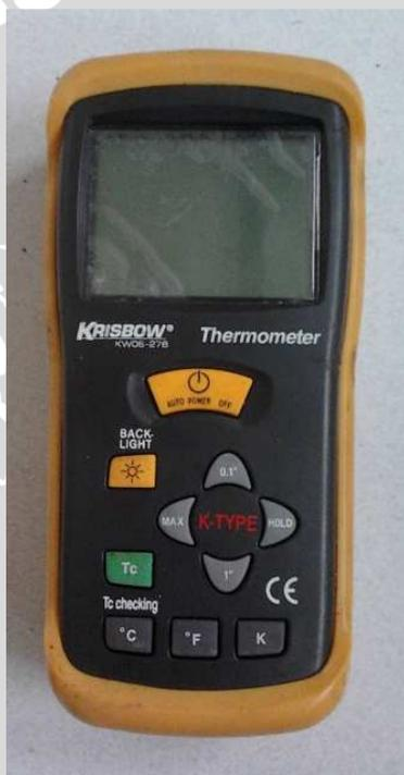
Gambar E. Digital thermocouple
