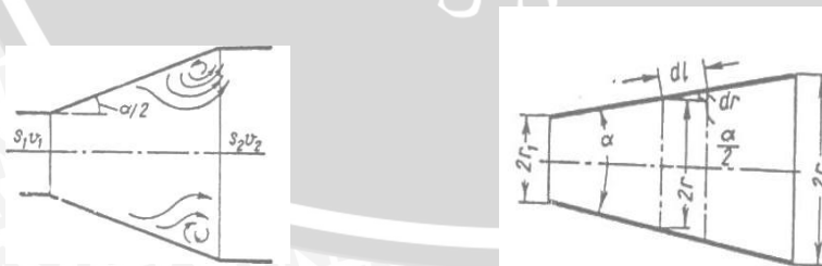
a. Eddy formation in a diffuser
