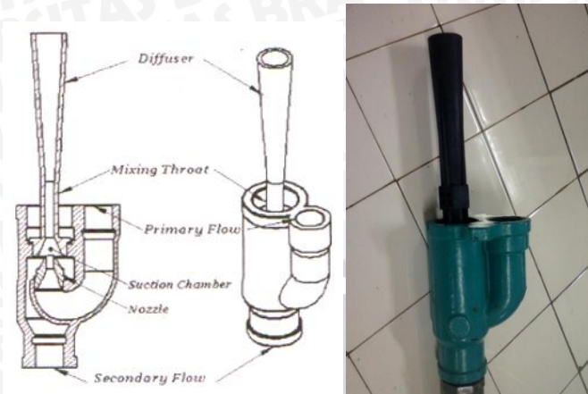
Gambar 3.2: Jet pump
