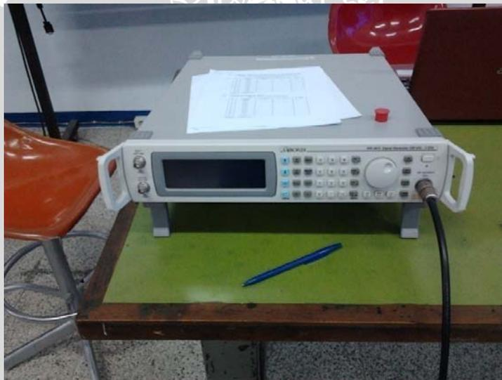
Gambar 11 *Signal Generator FR 3413 250kHz – 3 GHz Aeroflex*
