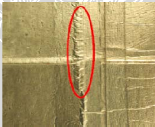
Gambar 2.5 Defect of LS Sumber : PT. Greenfields Indonesia
