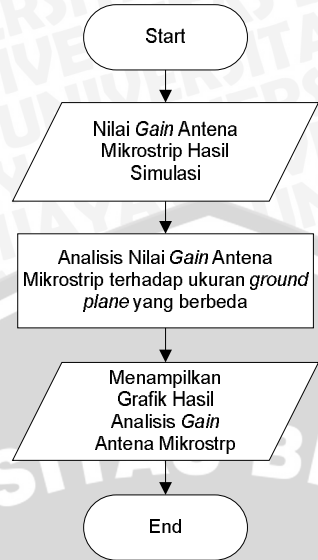
Gambar 3.6 Diagram Alir Perhitungan Gain Antena Microstrip
