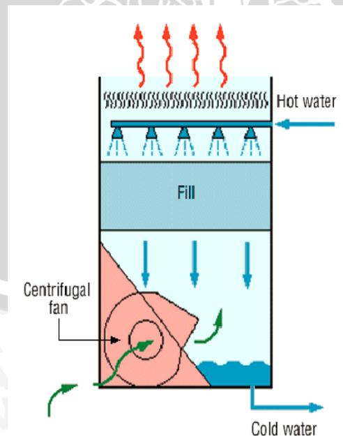
Gambar 2.3. *Forced draft Cooling tower*.
