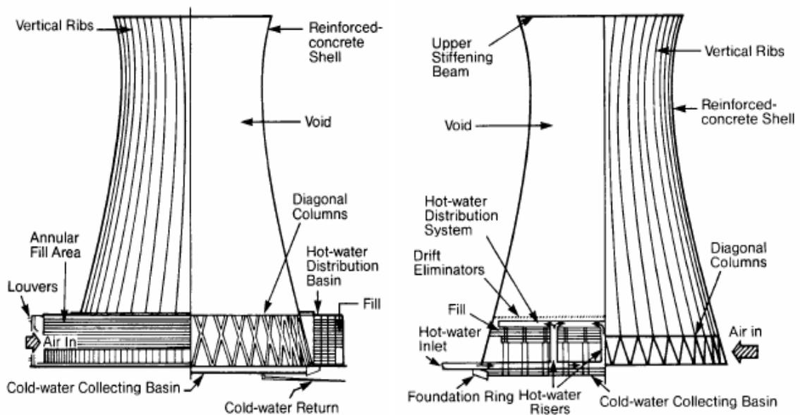
Gambar 2.4. *Natural Draft cooling tower* aliran melintang.
