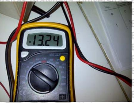
Gambar 5.20 Pengukuran Adaptor driver relay starter
