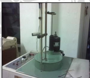
Gambar 3.2 *bomb calorimeter*
