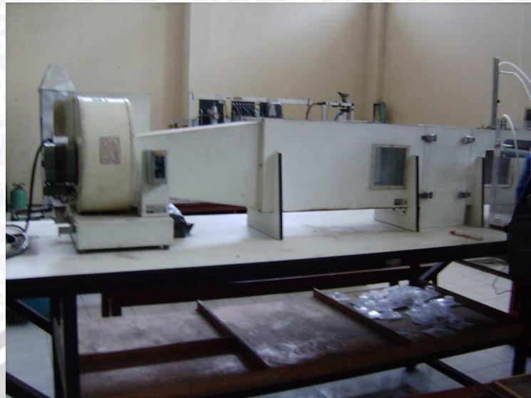
Gambar 3.1: *Wind Tunnel*
