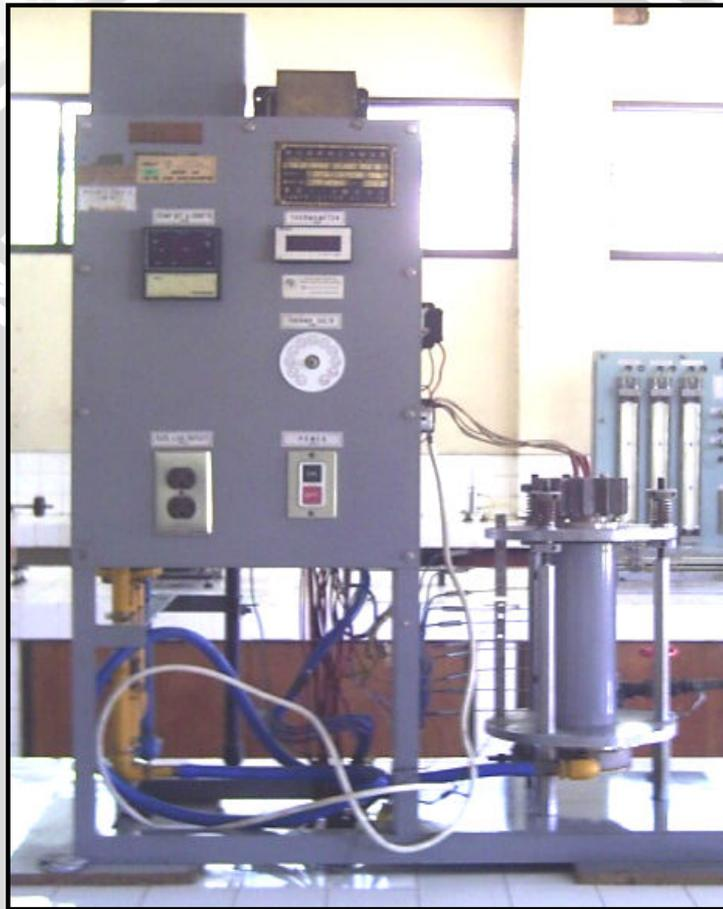
Gambar. 3.2. Thermal Conductivity Measuring Apparatus
