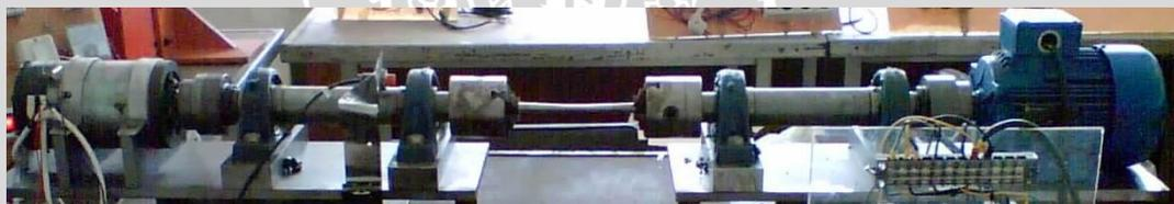
Gambar 3.1. *Rotary Bending Machine*
