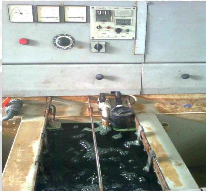
Gambar 3.4 Bak elektroplating nikel
