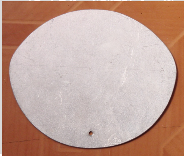
Gambar 4.10 Hasil fabrikasi antenna Rugby Ball
