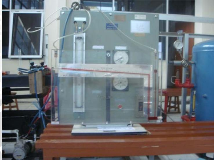
Gambar 3.2: *Inclined Manometer*
