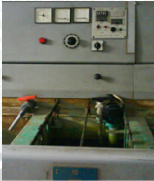
Lampiran 10. Gambar Instalasi Elektroplating
