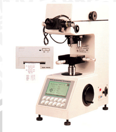
Gambar 2.5: Alat Uji Kekerasan Micro Vickers Hardness Sumber: www.metalkorea.or.kr/Measurable/...cro.html
