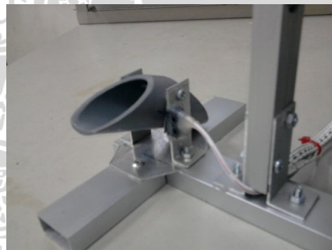
Gambar 4 Pemodelan sensor curah hujan (Tipping Bucket)
