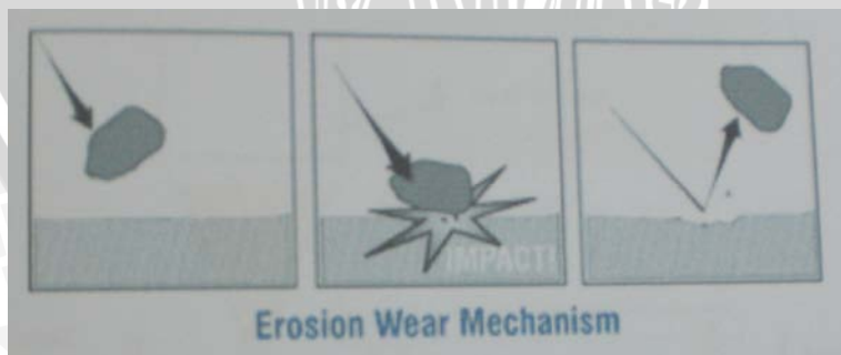
Gambar 2.16 Erosion Wear (Sumber : Robert Scot, 2008)
