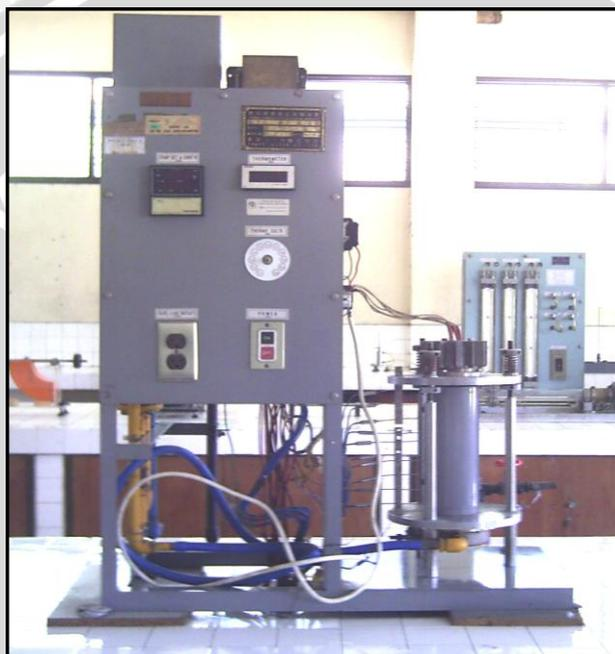
Gambar. 3.2. *Thermal Conductivity Measuring Apparatus*
