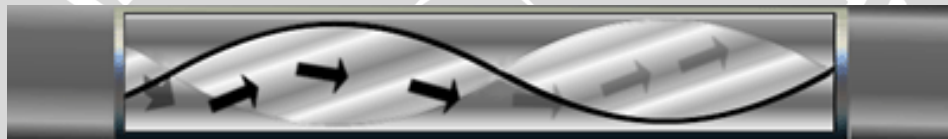
Gambar 2.17 : Static twisted tape Sumber : http://www.alcotwin.com/products.html
