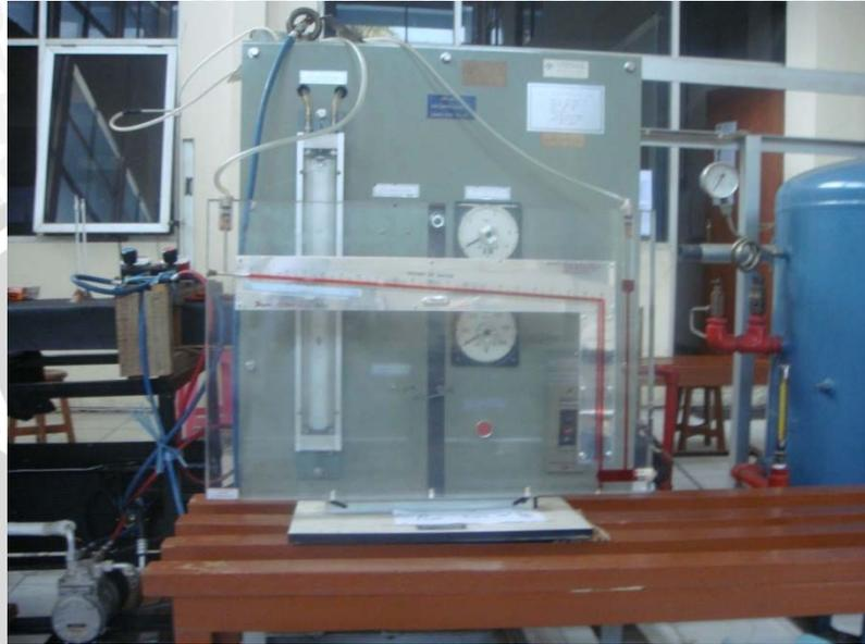
Gambar 3.2: *Inclined Manometer*
