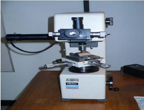
Alat Uji Kekerasan Mikro Vickers
