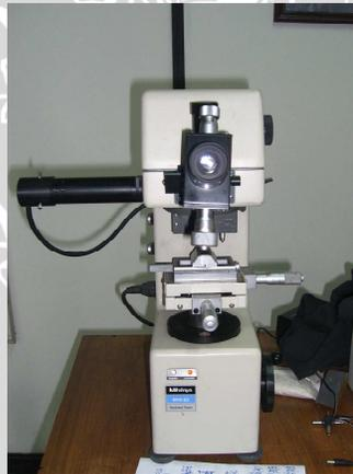
Gambar 2.4. *Micro Vickers Hardness Tester type Mitutoyo MVK-E3*
